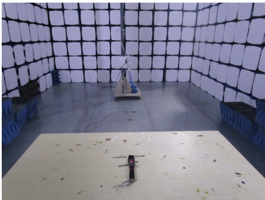
Radiation Emission Test Setup (30MHz to 1GHz)
