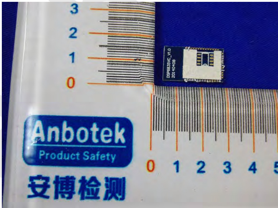
Figure 15 PCB of the EUT-Back View
