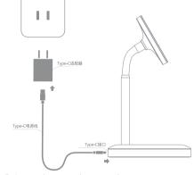
Connect the power adapter to socket.
