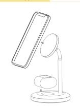
When the wireless charger is connected to an ordinary 5V adapter through Type-C to Type-C cable (Standard cable for this product) or USB-A to USB-C cable, the product works in ordinary wireless charging mode and only supports single 5W load. If you use QC , PD standard adapter, the product will works in quick wireless charging mode and supports 7.5W/10W/15W load.
