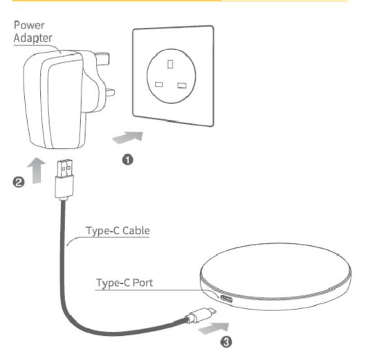
① Connect the power adapter to socket.
