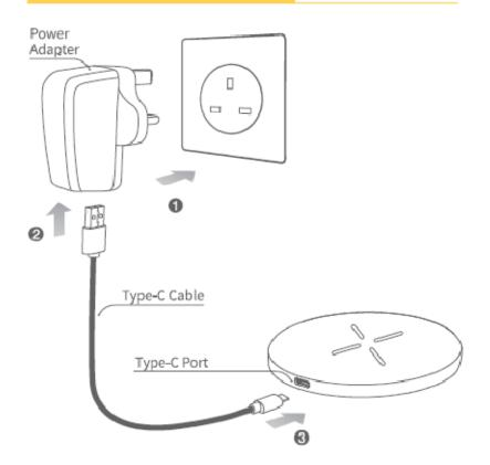
Connect the power adapter to socket.
