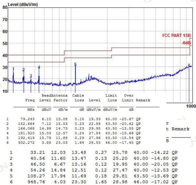
Remark: Absolute Level = Reading Level + Factor, Margin = Absolute Level – Limit Factor = Ant. Factor + Cable Loss – Pre-amplifier Remark:
