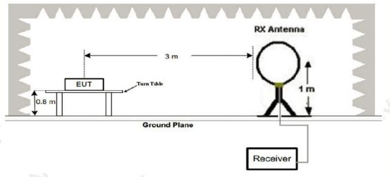
2. Radiated Emission Test-Up Frequency 30MHz~1GHz
