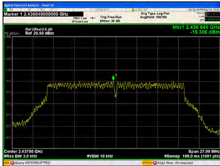
ANT1 TX 11n HT20 Middle channel
