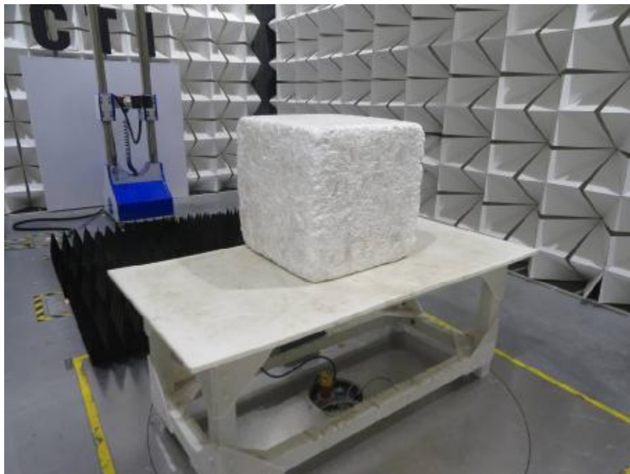
Radiated spurious emission Test Setup-2(Above 1GHz)
