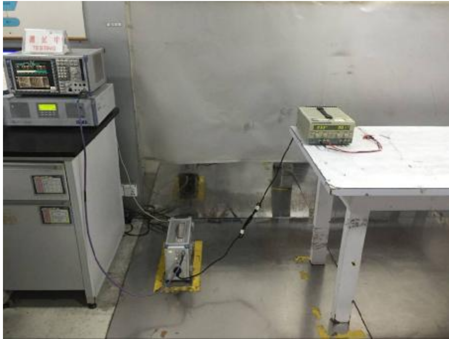
Conducted Emissions Test Setup
