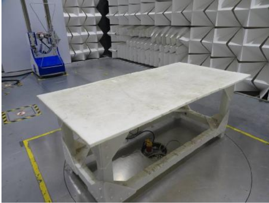
Radiated spurious emission Test Setup-1(Below 1GHz)
