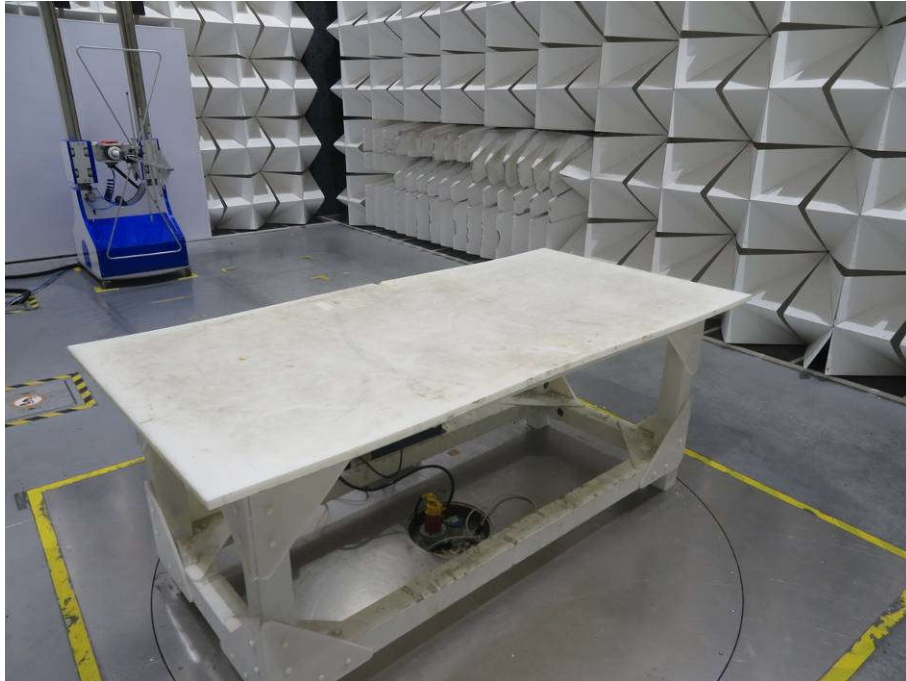
Radiated spurious emission Test Setup-1(30MHz-1GHz)
