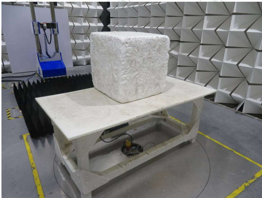
Radiated spurious emission Test Setup-2(Above 1GHz)
