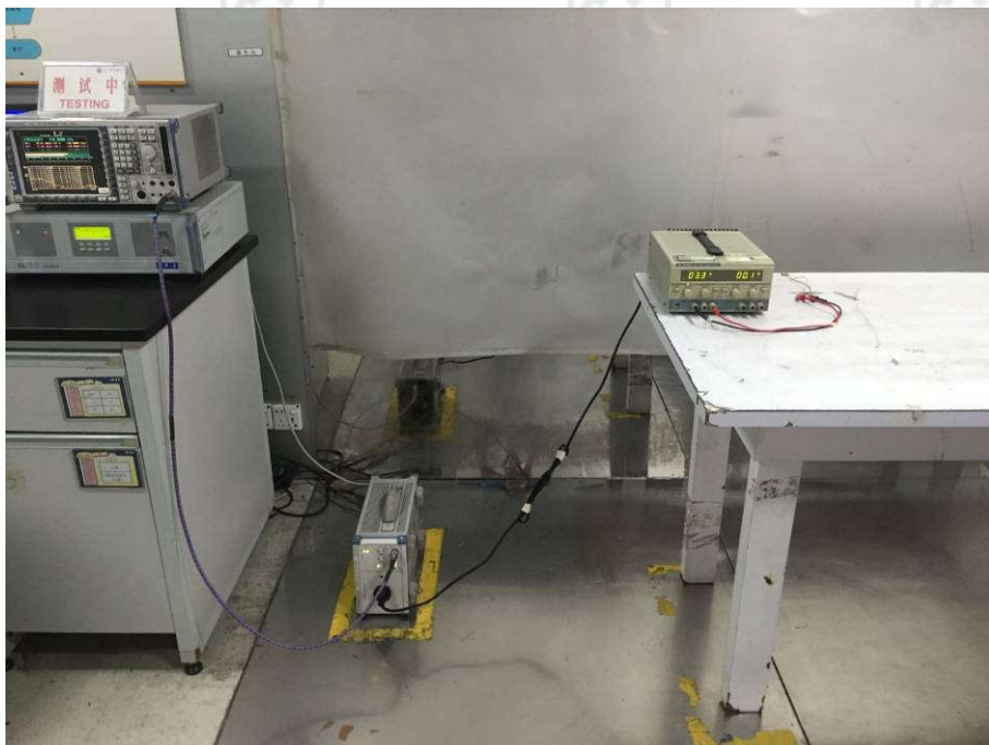
Conducted Emissions Test Setup
