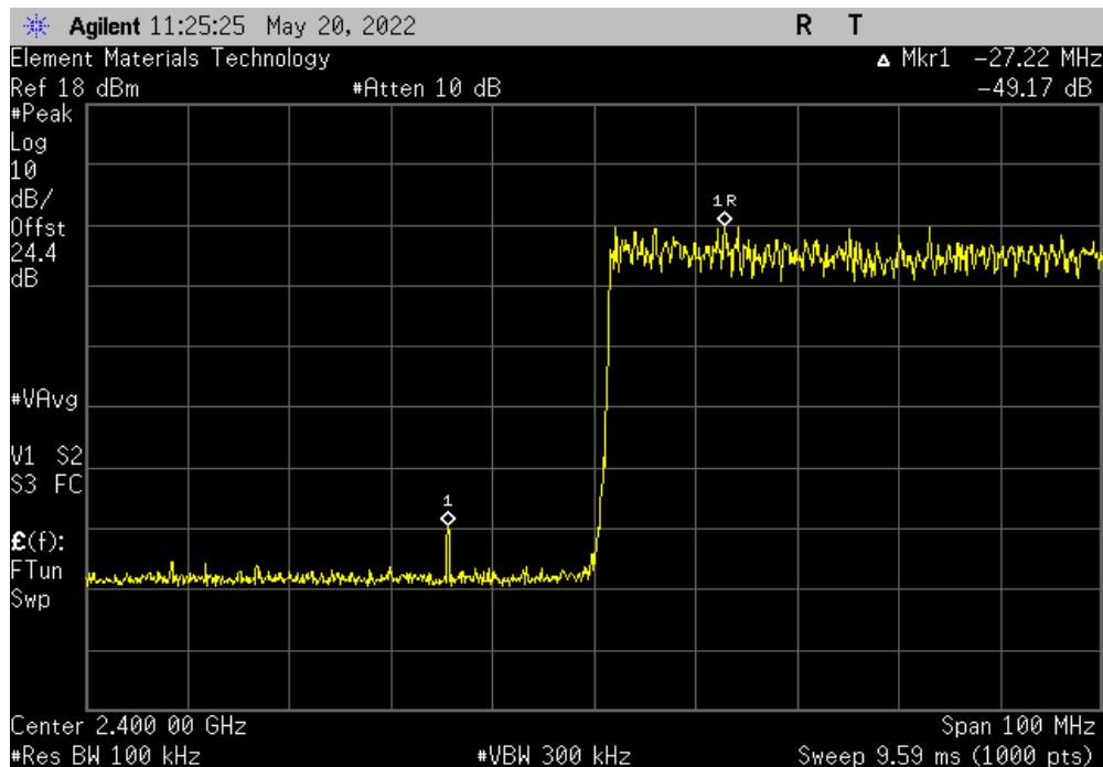
Hopping Mode (All Channels), 3DH5, 8-DPSK, High Channel, 2480 MHz
