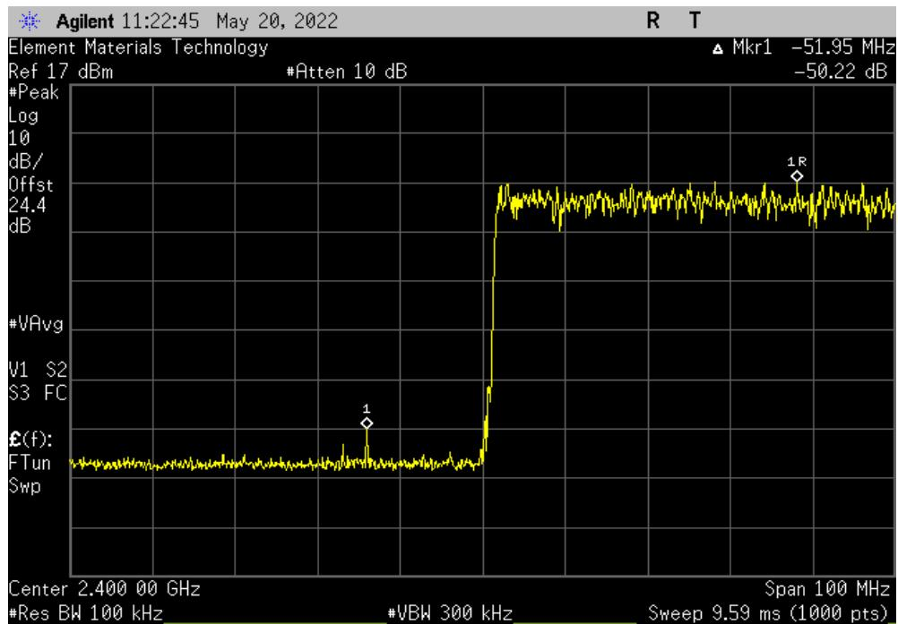
Hopping Mode (All Channels), 2DH5, pi/4-DQPSK, High Channel, 2480 MHz
