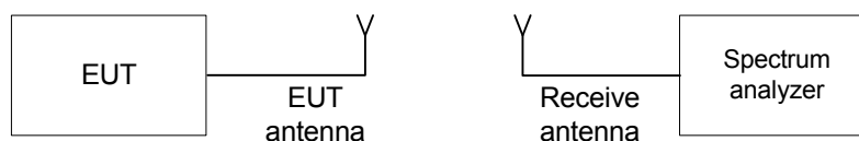
Figure 7.4.1 Band edge emission test setup
