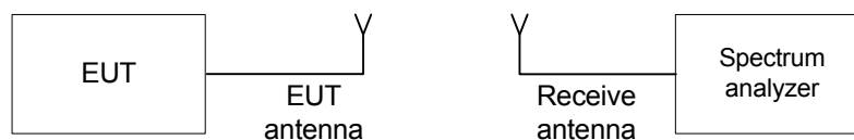
Figure 7.1.1 The 6 dB bandwidth test setup
