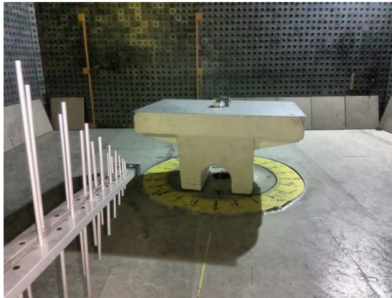
Photograph 8.1.1 Setup for radiated emission measurements
