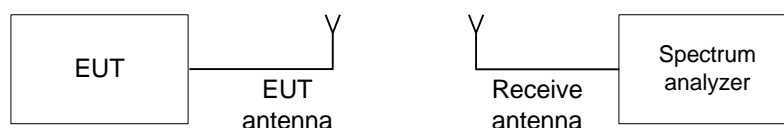
Figure 7.3.1 Occupied bandwidth test setup
