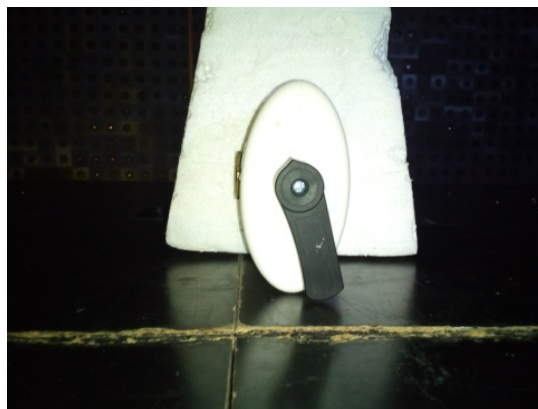
Photograph 6.4.3 EUT in Z-axis orthogonal position
