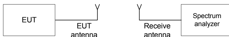
Figure 7.3.1 Occupied bandwidth test setup
