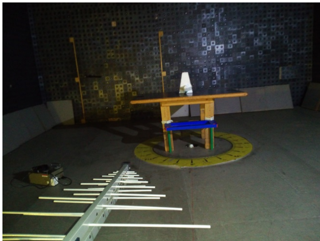
Photograph 8.1.1 Setup for radiated emission measurements
