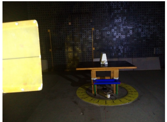
Photograph 8.1.1 Setup for radiated emission measurements
