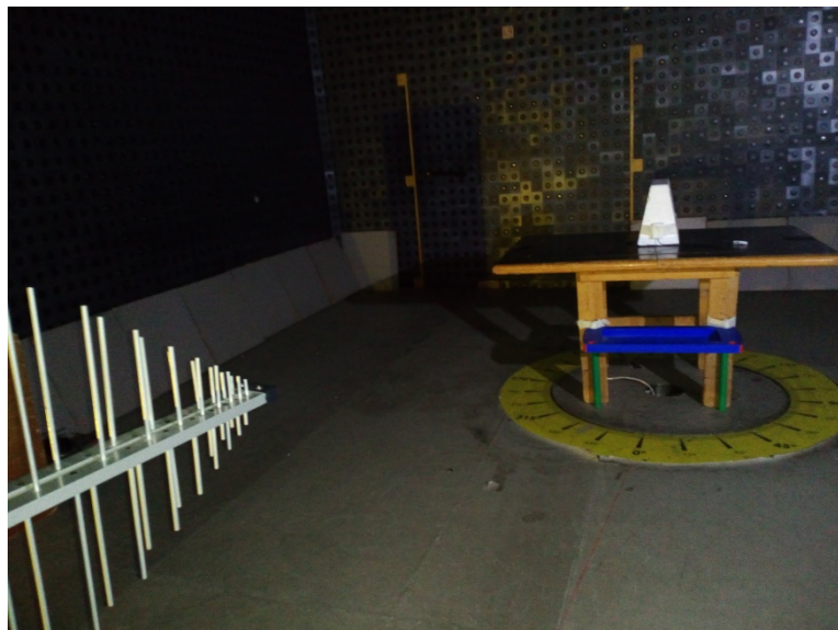
Photograph 8.1.1 Setup for radiated emission measurements
