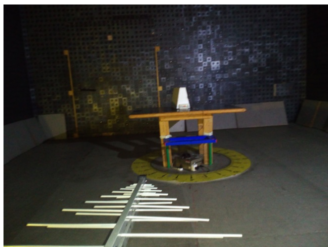
Photograph 8.2.1 Setup for radiated emission measurements, general view
