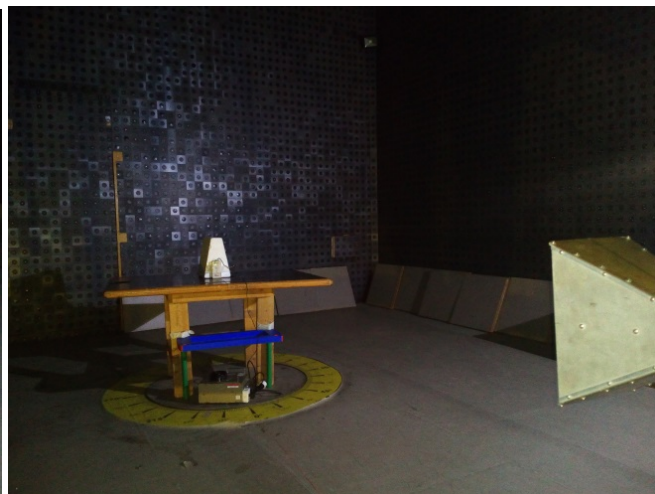
Photograph 8.2.1 Setup for radiated emission measurements, general view
