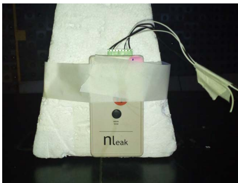
Photograph 8.2.2 Setup for radiated emission measurements, EUT cabling
