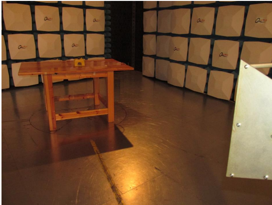
Photograph 3- Radiated spurious emission measurements 1 GHz – 6 GHz test setup
