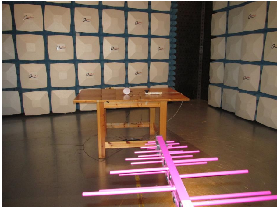
Photograph 3- Radiated spurious emission measurements above 30 MHz – 1 GHz test setup
