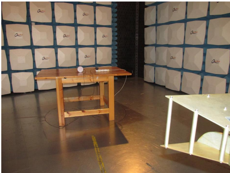
Photograph 4- Radiated spurious emission measurements 1 GHz – 6 GHz test setup
