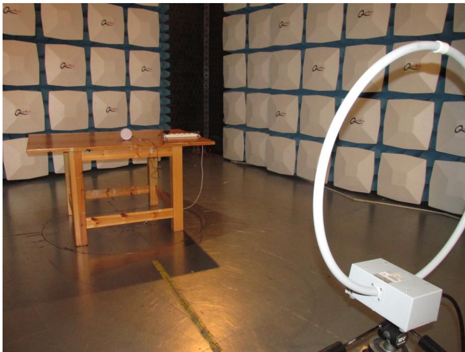
Photograph 2 –Radiated spurious emission measurements below 30 MHz test setup
