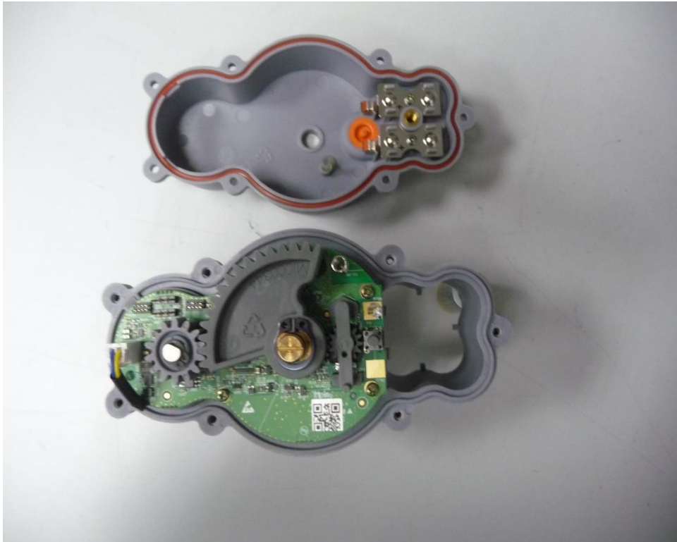
Photograph No.1 Actuator shut off unit internal view
