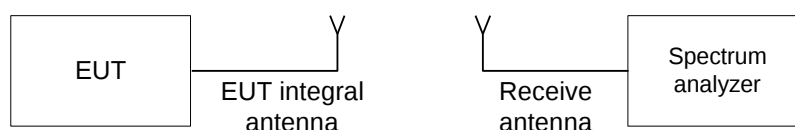
Figure 7.1.1 Setup for transmitter shut down test
