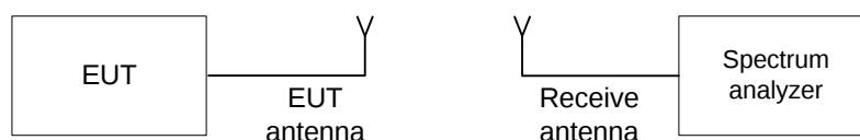
Figure 7.3.1 Occupied bandwidth test setup
