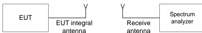
Figure 7.1.1 Setup for transmitter shut down test
