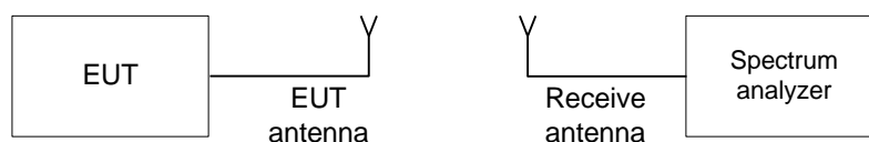
Figure 7.3.1 Occupied bandwidth test setup
