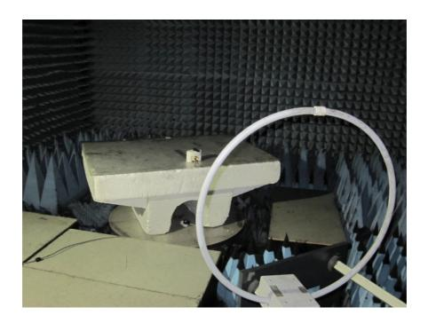
Photograph No.2 Setup for carrier, spurious emission field strength measurements in the anechoic chamber in 30 - 1000 MHz range
