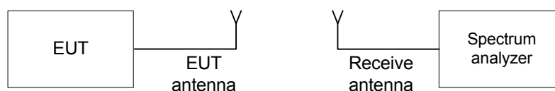
Figure 7.3.1 Occupied bandwidth test setup
