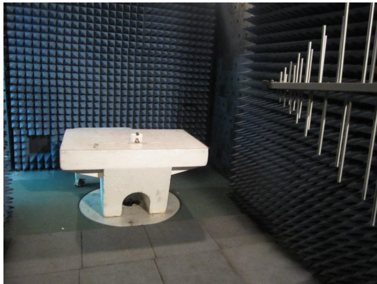
Photograph 8.1.1 Setup for radiated emission measurements
