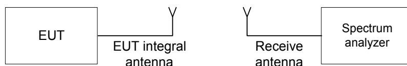
Figure 7.1.1 Setup for transmitter shut down test
