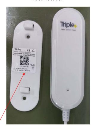
Label with **FCC ID:2AFOICLMFLD10** and **IC:20798-CLMFLD10** is located at the bottom side of the Flood detector. The statement according to FCC part 15 §15.19(a)(3) is placed in User's Manual, page 26 (Application exhibit User\_manual\_28548).
