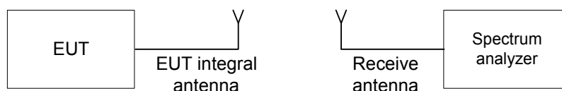
Figure 7.1.1 Setup for transmitter shut down test
