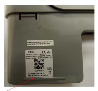
Label with FCC ID:2AFOICLMCTRL10 and IC:20798-CLMCTRL10 is located at the bottom side of the HUB. The statement according to FCC part 15 §15.19(a)(3) is placed in User's Manual, page 26 (Application exhibit User\_manual\_28549).
