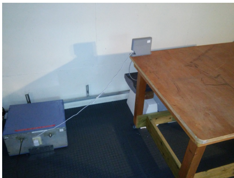
Photograph 8.1.1 Setup for conducted emission measurements
