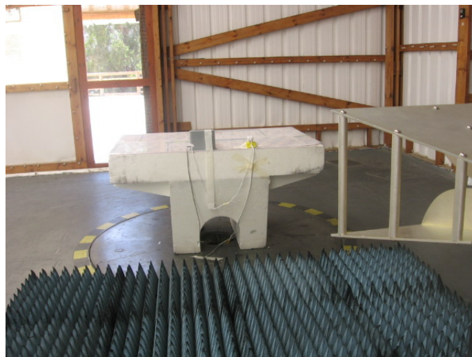
Photograph 8.2.2 Setup for radiated emission measurements, general view
