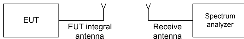
Figure 7.1.1 Setup for transmitter shut down test
