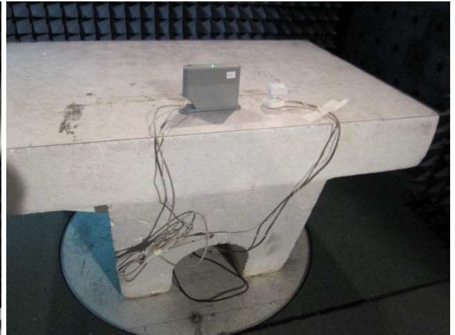
Photograph 8.2.1 Setup for radiated emission measurements
