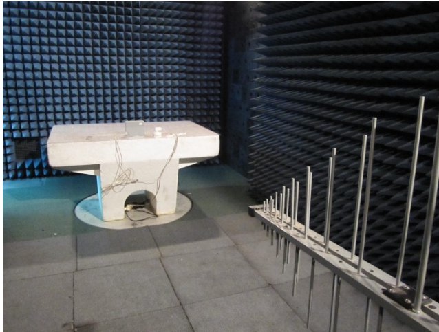
Photograph 8.2.1 Setup for radiated emission measurements
