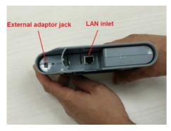
4. Position the HUB on its permanent location. For wall mounting, bring the HUB's rear mounting pins close to the wall and gently slide it down the wall mount's dimples. Please do not attempt to rotate the HUB on the mounting in order to avoid physical damage to the enclosure.
