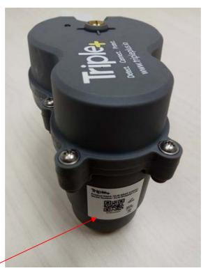
Label with FCC ID:2AFOICLMASOU20 and IC:20798-CLMASOU20 will be located at the bottom part of the unit's shell, on the motor cover. The statement according to FCC part 15 §15.19(a)(3) is placed in User's Manual, page 26 (Application exhibit User\_manual\_29189).
