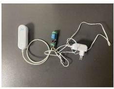
CBM-FDAMAP-5: Flood Sensor device. Power capabilities – powered by 2x AAA batteries. RF connectivity by 915MHz radio.
