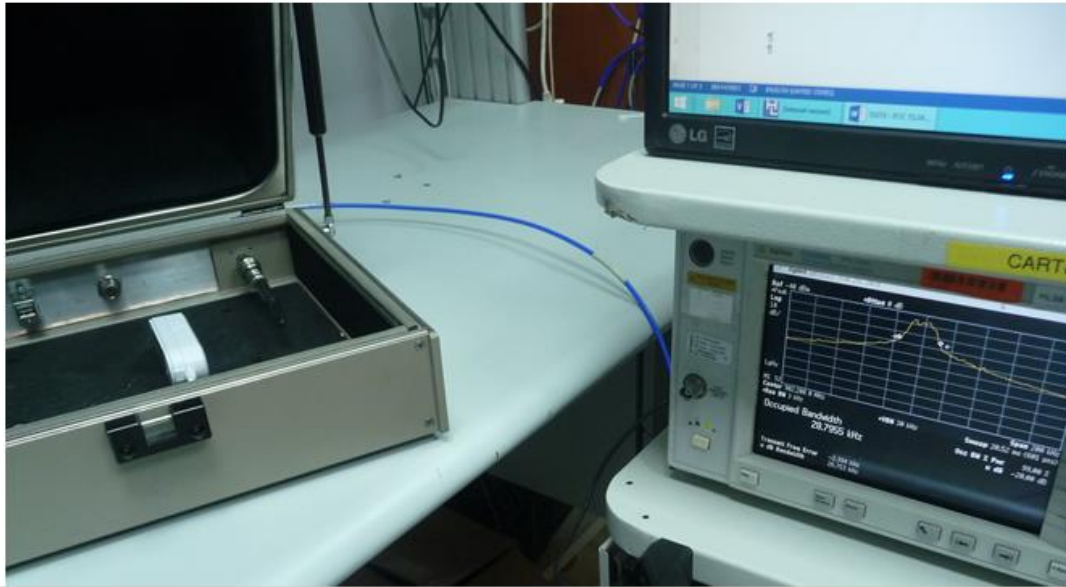
Photograph No.4 Setup for 20 dB bandwidth measurements
