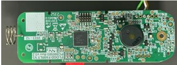
Photograph No.9 Flood family (Universal Switch) Model Name CBM-PSAMAP-5 unit internal view
