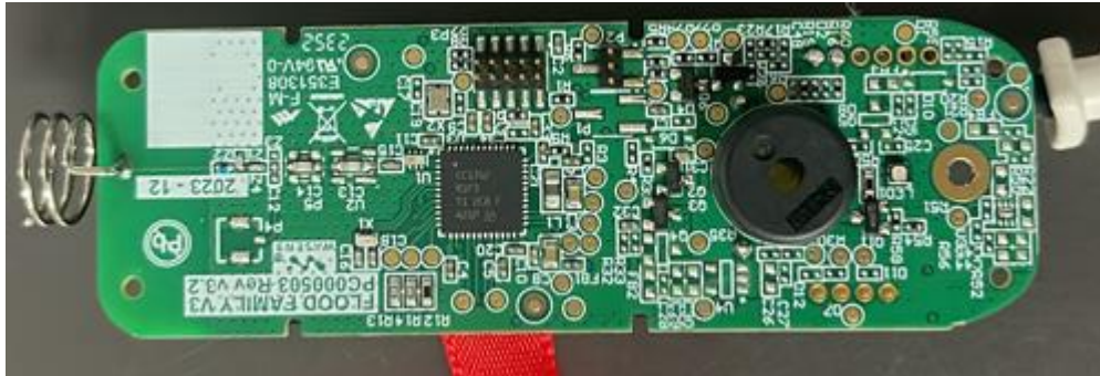
Photograph No.5 Flood family (Universal Switch) Model Name CBM-SRAMAP-5 unit internal view
