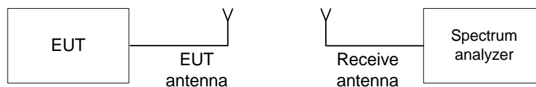
Figure 7.2.1 Carrier frequency separation test setup
