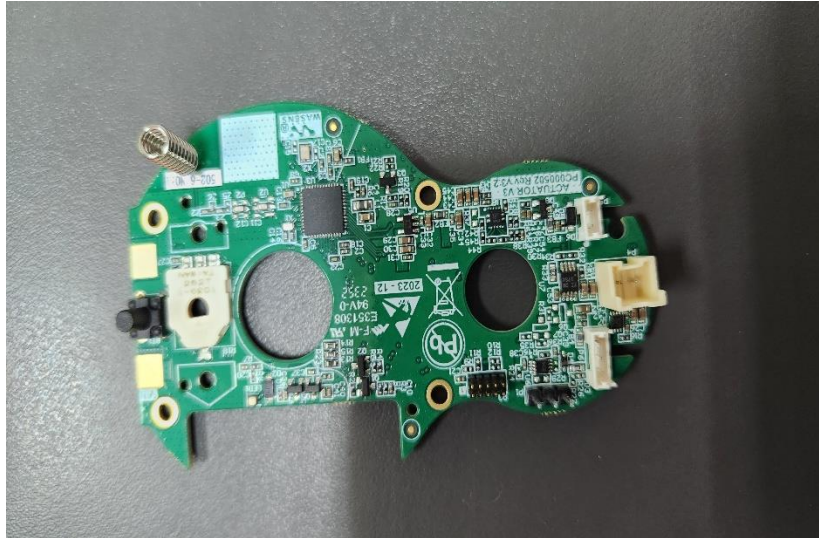
Photograph No.1 Shut Off Actuator unit internal view
