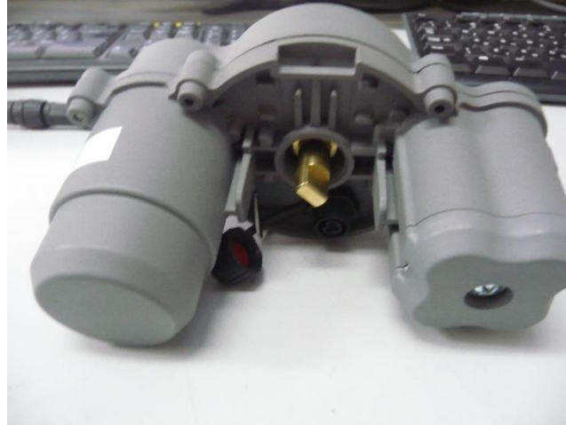
Photograph No.2 Shut Off Actuator unit bottom view
