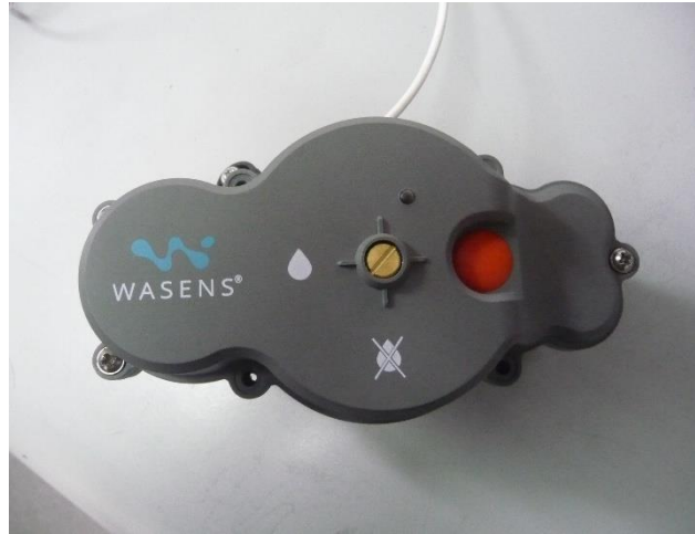
Photograph No.1 Shut Off Actuator unit front view
