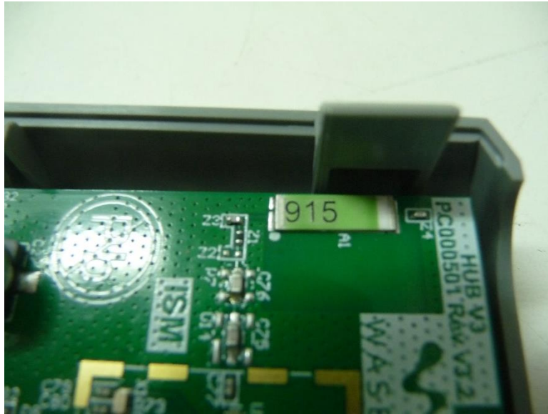
Photograph No.5 Controller unit antenna
