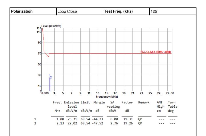
Note 1: Emission Level (dBuV/m) = SA Reading (dBuV/m) + Factor (dB)
