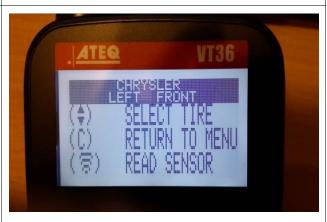
Hold the VT36 directly on the rubber tire, over the valve stem.
