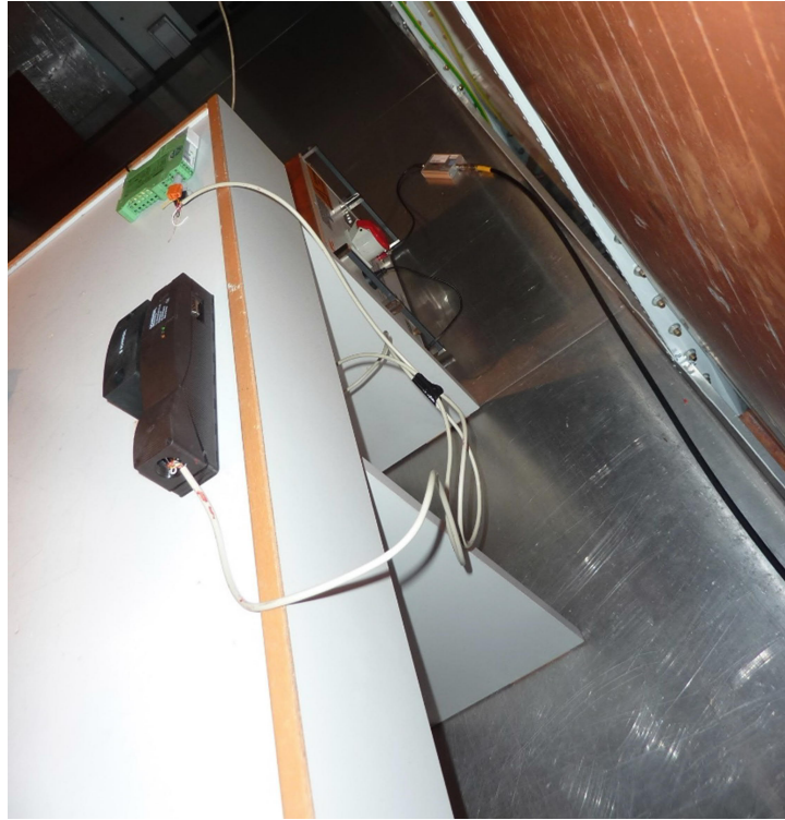
191513SK_05: Conducted measurement 150 kHz – 30 MHz
