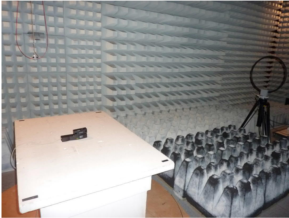
191513SK_01: Preliminary measurement H-Field 9 kHz – 30 MHz
