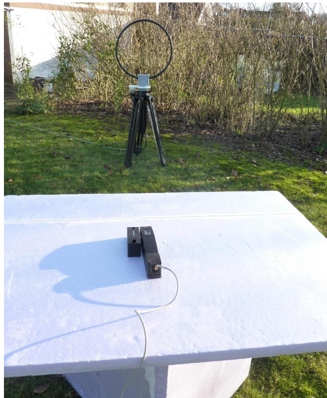
191513SK_02: Final measurement H-Field 9 kHz – 30 MHz
