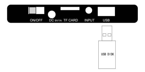
Input USB disk under power on status, change to USB play status automatically. Input USB disk under power off status, need short press mode key to change to USB play status after power on.
