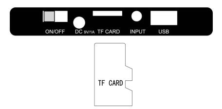
Input TF card under power on status, change to TF play status automatically. Input TF card under power off status, need short press mode key to change to TF play status after power on.
