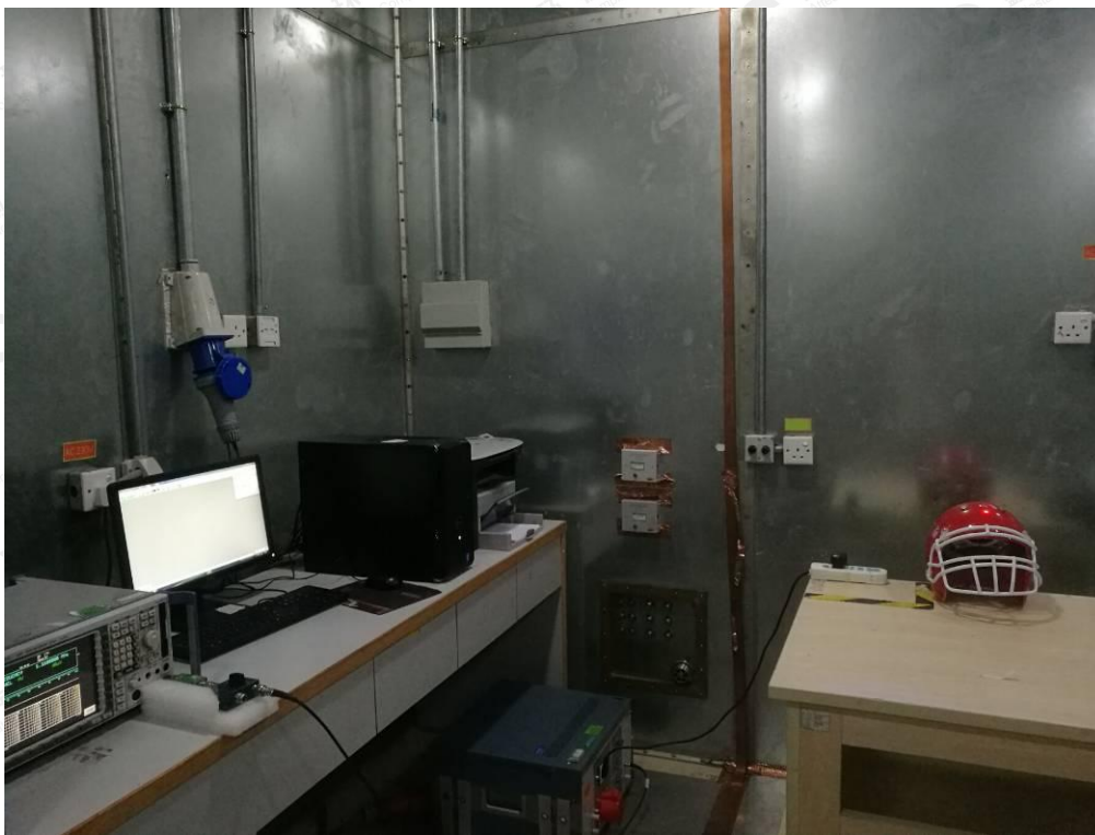
FCC RADIATED EMISSION TEST SETUP
