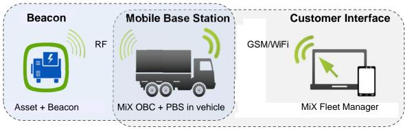
Communicator OBC to convert the vehicle to a Mobile Base Station (MBS)
