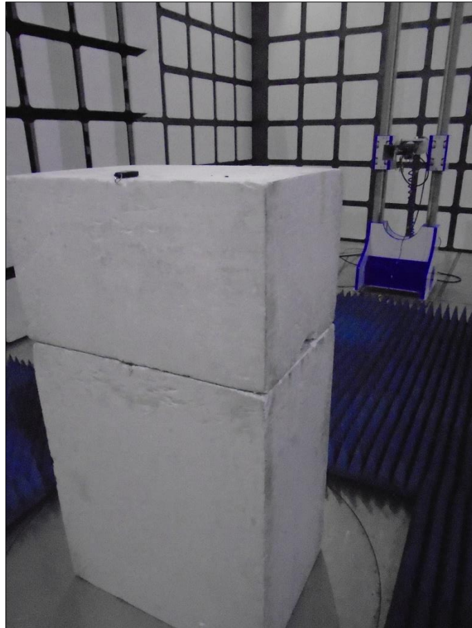
Figure 69 - Test Setup - 1 GHz to 18 GHz - X Orientation
