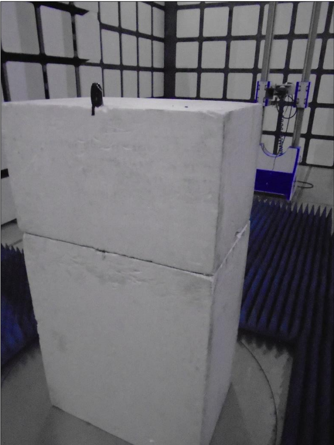
Figure 70 - Test Setup - 1 GHz to 18 GHz - Y Orientation
