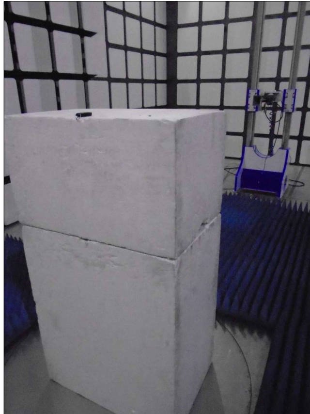
Figure 69 - Test Setup - 1 GHz to 18 GHz - X Orientation
