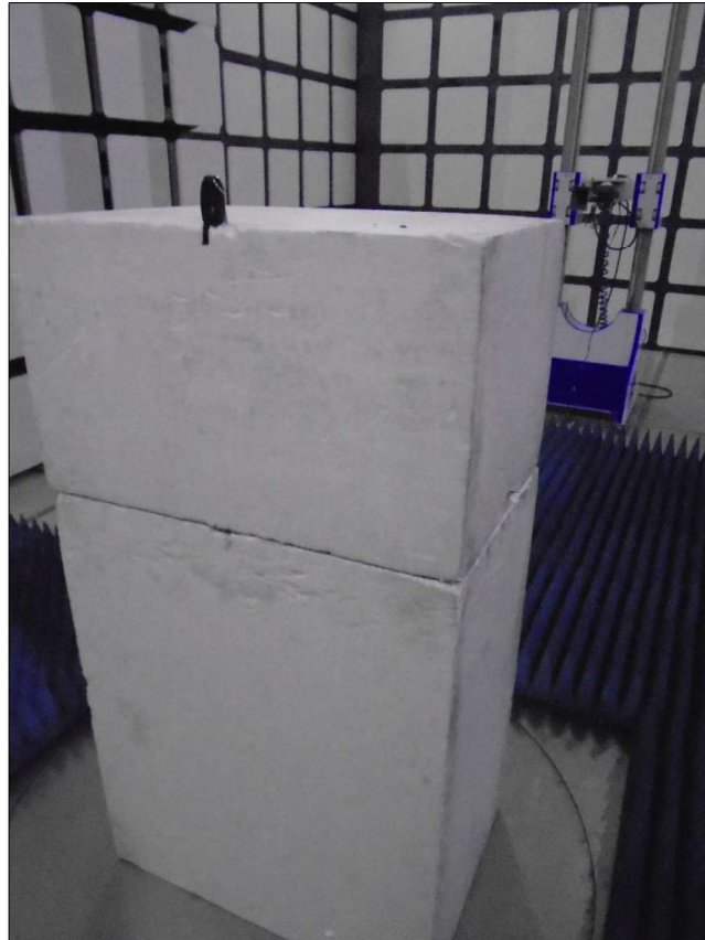
Figure 70 - Test Setup - 1 GHz to 18 GHz - Y Orientation
