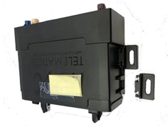
Figure 13: Attach the clips by sliding them over the brackets on the unit.
