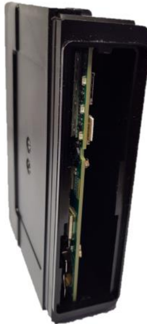
Figure 4: Insert the SIM card into the correct SIM card slot; ensure it is fully seated (clicks into place).
