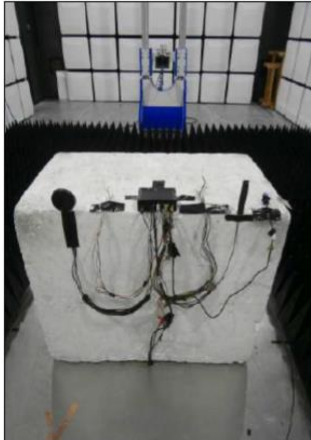
Figure 23 - Test Setup - 1 GHz to 14 GHz - X - Orientation
