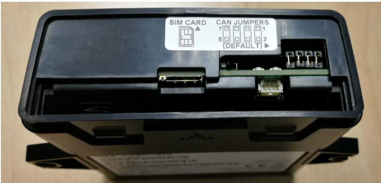
Figure 1: Picture of the MiX 46MC-4G (back plate removed)
