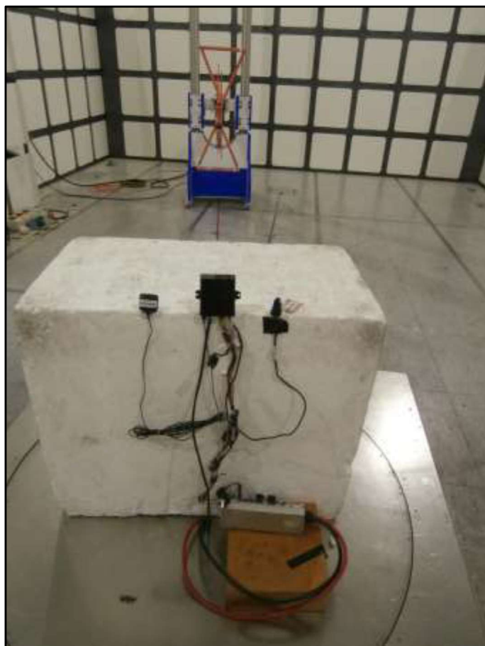
Figure 60 - Test Setup - 30 MHz to 1 GHz – Y Orientation
