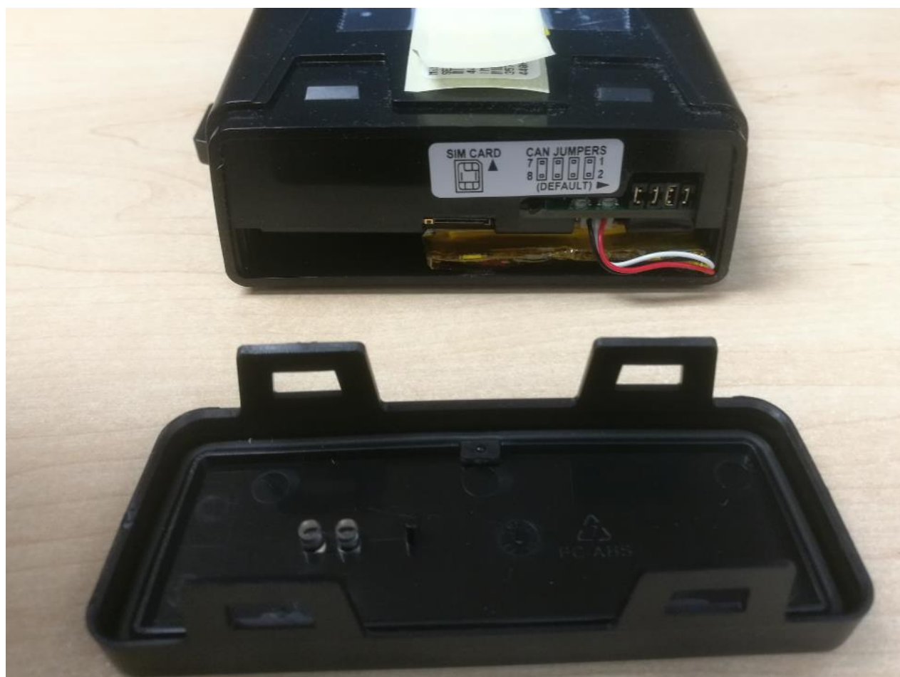
Figure 10: View of MiX 460C-4G-B with Rear Panel Removed (backup battery inserted)
