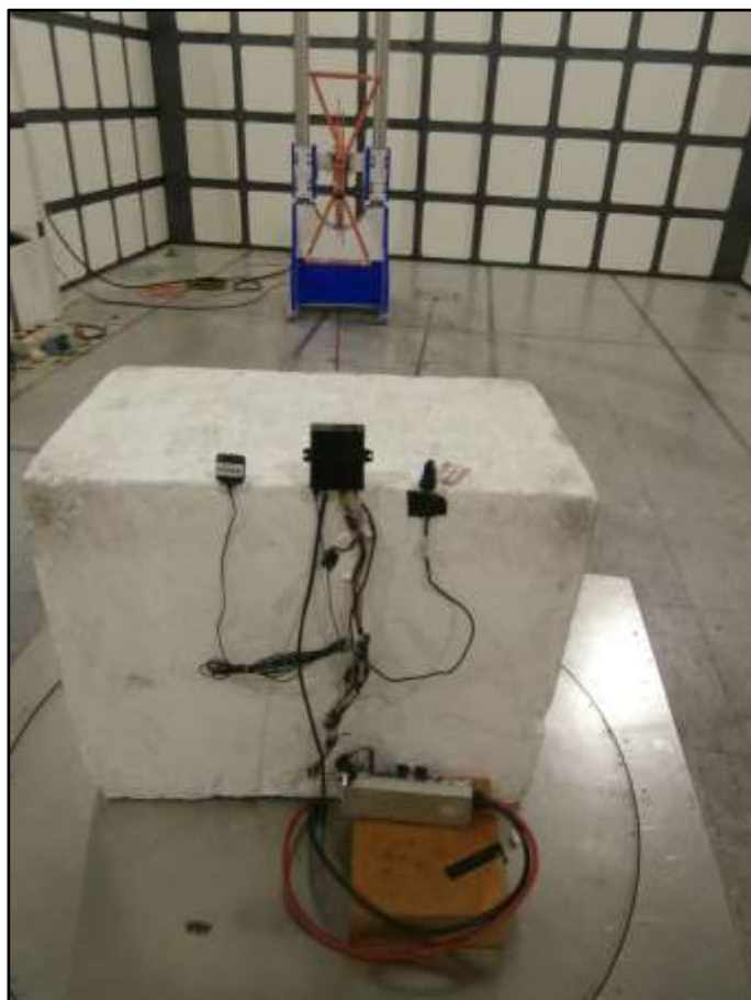
Figure 60 - Test Setup - 30 MHz to 1 GHz – Y Orientation
