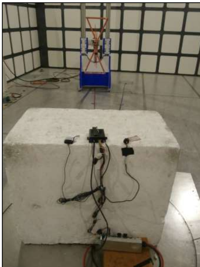
Figure 59 - Test Setup – 30 MHz to 1 GHz – X Orientation
