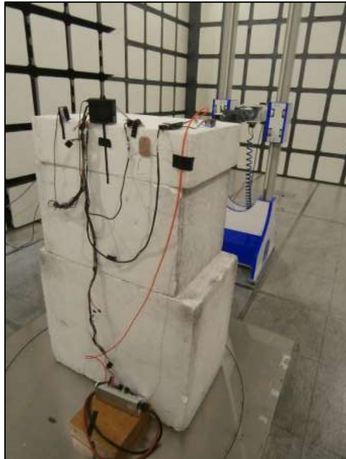
Figure 67 - Test Setup - 18 GHz to 25 GHz – Z Orientation
